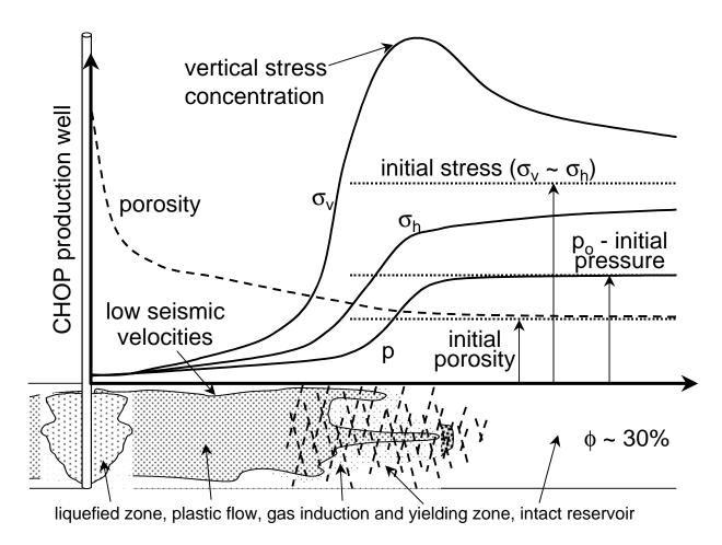
Fig 1: Stresses, pressures and porosities around CHOP wells
